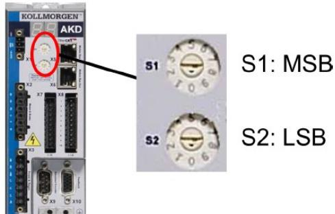
The rotary switches on the front of the AKD (S1&S2) correspond to the CAN node address.
