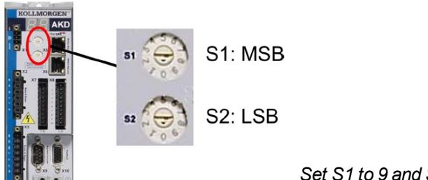
2. Push the button B1 on the AKD for at least 3 seconds until the rotary switch setting is displayed on the AKD-display.
