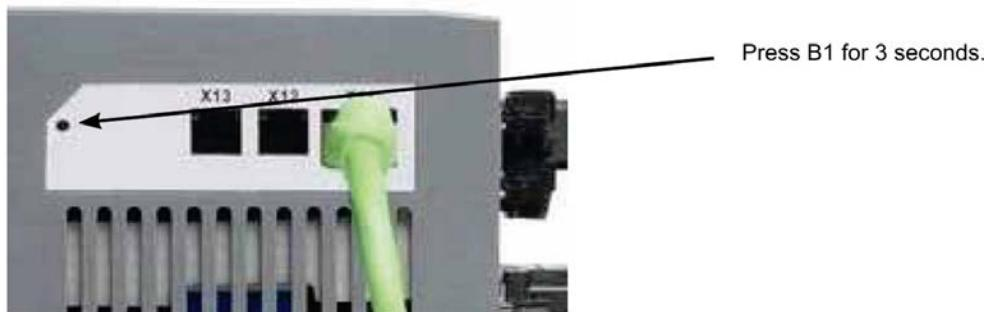
The seven segment display shows **Cn** during the process of changing DRV.TYPE to CAN.
