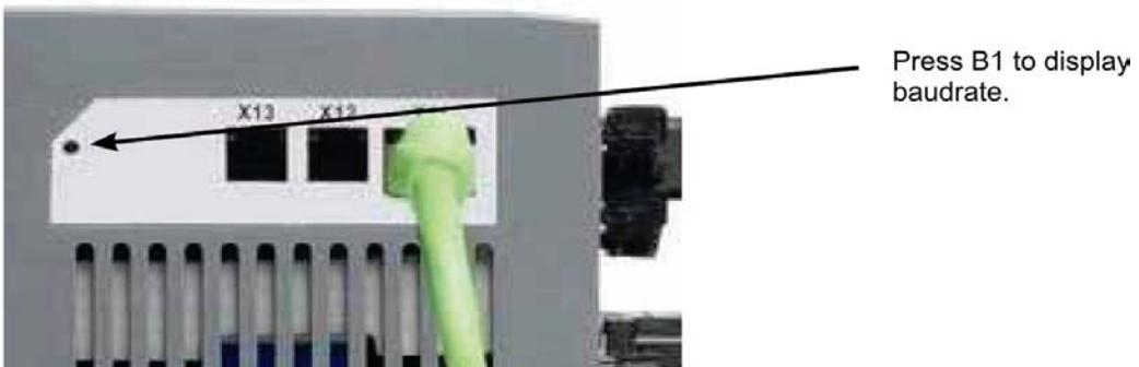
3. When the display blinks with the set rotary switch setting stop pushing B1 and wait until the blinking stops. During that time the parameter FBUS.PARAM01 is set to the new value and all parameters are stored to the non volatile memory. The new setting will be taken with the next power-up of the drive.
