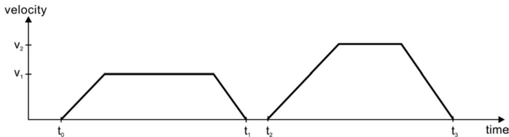
With change\_set\_immediately set to "1" (6), the host instructs the drive to apply a new setpoint immediately after reaching the previous one. The relative timing of the other signals is unchanged. This behavior causes the drive to process the next setpoint X2 in advance, and to hold its velocity when it reaches the target\_position X1 at t1. The drive then moves immediately to the next target\_position X2 that has already been calculated.
